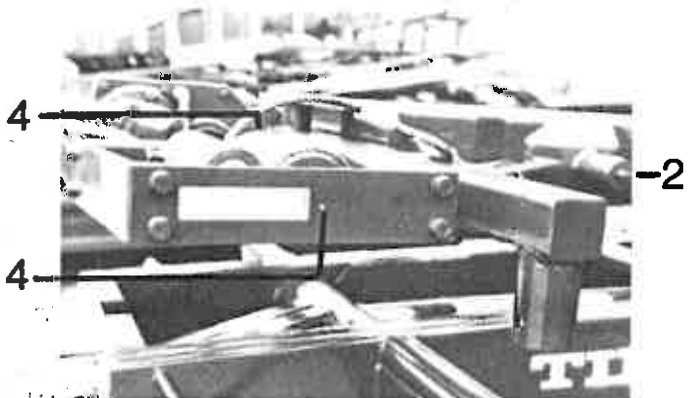
Fig. 9. Fedtsmøring Grease lubrication
